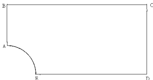
Figure 1. Quarter plate model of C–C composites with a central circular hole.
